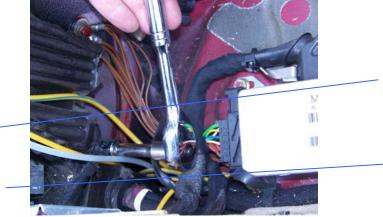
To be on the safe side, you can tape the 14-mm hex bolt to your socket once it has been almost unscrewed, and tape the socket to the ratchet's extension. **or better yet**, **stick rags into all holes that you could accidentally drop the bolt into while pulling it out.** This would be a safeguard against the bolt accidentally falling into the rocker panel,
