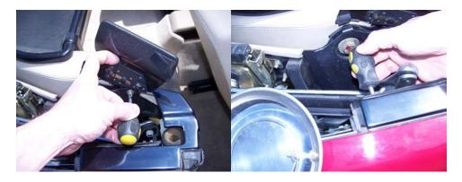
Remove the Phillips screw holding the rear compartment trim panel.
