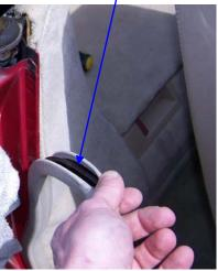
Release the rubber molding from the top case plate with a flat screwdriver. (May not be necessary in newer models.)
