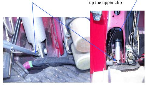
Put a rag under the lower hydraulic line, pull out the hydraulic lines and pull out the cylinder. The cylinder has a rubber boot attached to it. It is tied on with a tie wrap. Either cut the tie wrap, or gently slide the cylinder out of the boot with the tie wrap in place. If you want to take out the boot with the cylinder, pull the drain hose upward out of the chassis and maneuver the hydraulic line through the cutout in the boot first. Wrap the cylinder in a rag.
