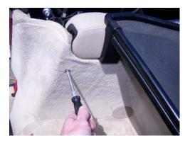
Remove the rear compartment side trim panel – take a look at the photo below first, showing how the panel is fastened. Start pulling from the upper outer corner, locate all the fasteners and pull near their position, then lift up the panel out of the hook in the rear top. It is best to have the roll bar in the raised position for this; removal of the windscreen is optional.
