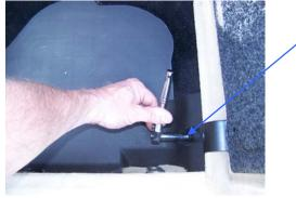
Find the 14-mm hex head for the main cylinder's bottom bolt. It is below (not behind) a bunch of wires and foam rubber. Start on the passenger side and try to gain the same perspective as shown in the photo below – roughly follow the front edge of the controller module all the way to the outer edge of the compartment.
