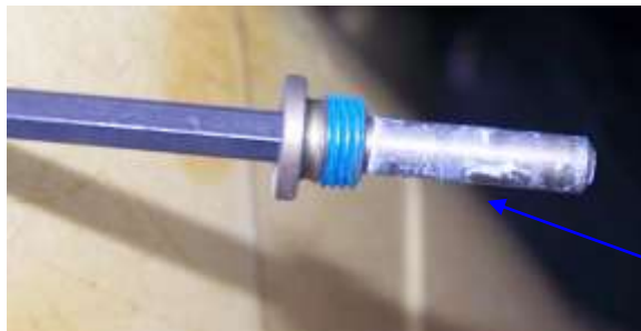
(Front pin/bolt with Allen head for '90-'95 models)
